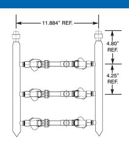
INSTALLATION NOTE: MANIFOLD MUST BE MOUNTED A <u>MINIMUM</u> OF 2-3/4 INCHES FROM FACE OF WALL TO ALLOW FOR CLEARANCE OF SOLENOIDS.
