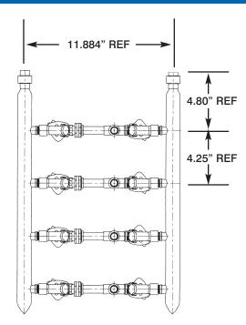
INSTALLATION NOTE: MANIFOLD MUST BE MOUNTED A <u>MINIMUM</u> OF 2-3/4 INCHES FROM FACE OF WALL TO ALLOW FOR CLEARANCE OF SOLENOIDS.
